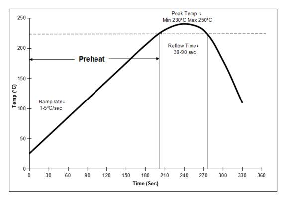
Reflow can be accomplished in a nitrogen controlled atmosphere at  $\leq$  100 ppm oxygen levels.
