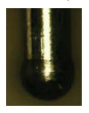
No Ball Defect After Reflow
