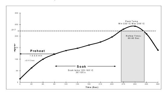
**Preheat Zone**- The preheat zone, is also referred to as the ramp zone, and is used to elevate the temperature of the PCB to the desired soak temperature. In the preheat zone the temperature of the PCB is constantly rising, at a rate that should not exceed 2.5 C/sec. The oven's preheat zone should normally occupy 25-33% of the total heated tunnel length.
