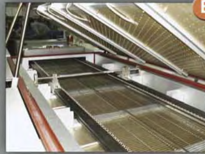
A Standard Combo Pin Chain Conveyor & Mesh Belt
