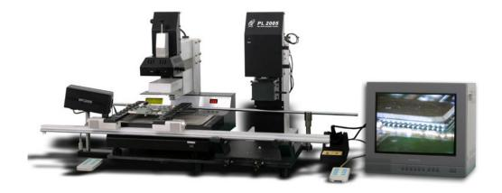
BGA rework system uses micro-processor control and infrared sensor technology to do soldering and desoldering to surface mounted components safely and accurately. It consists of QUALITEK IR2005 Infrared Rework System and QUALITEK PL2005 Precision Placement System.
